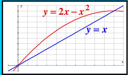
Solution: The points of intersection are given by  $x = 2x - x^{2}$   $\Rightarrow x^{2} - x = 0 \Rightarrow x(x-1) = 0$  $\Rightarrow x = 0 \text{ or } x = 1$
